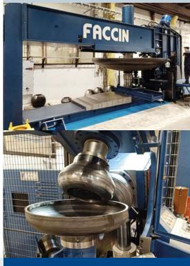
In the standard configuration, Faccin's BF flanging machines are equipped with automatic working cycle to assure the utmost ease of use during the flanging process even by inexperienced operators.
