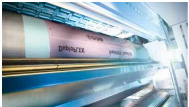
Fixing the final print layout on the printing cylinder on the flexo printing machine.
