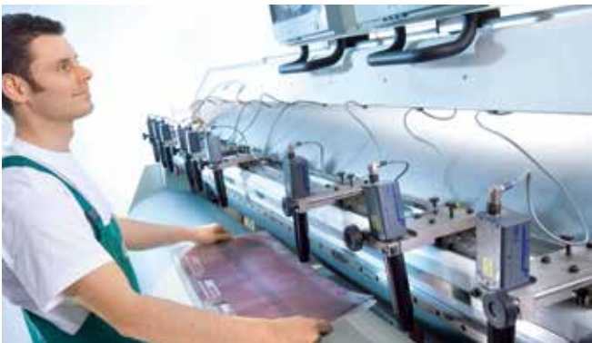
Digital plate mounting on PET with DuploFLEX® CB.
