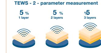
3 layers of the same material show the same moisture, the density is recognized and moisture results compensated  $\rightarrow$  correct results
