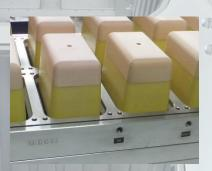
Superb rim surfaces thansk to cooled clamping frame
