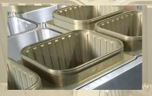
Hard Anodised and Teflon Coated forming surfaces for long lasting life and ease of shaping during forming process.
