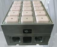
Motorised plug assists provides stretching control to the operator thus even material distribution is achieved easily.
