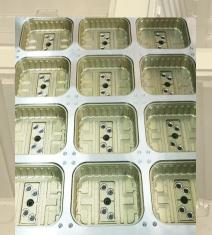
with magnet) facilitate change of inserts and saves down time during height changes. No need to take the mould out of the machine.
