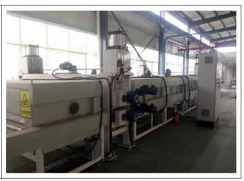
The machine could adopt the TPU /PVB /SGP/ EVA film laminating. Could choose the vacuum and pressure double function.
