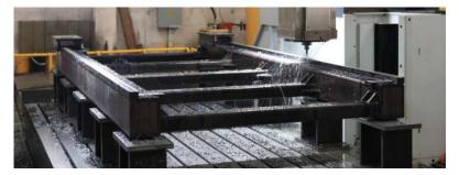
Main structure of double edger processed by annealing and aging treatment, then five sides are processed by CNC processing center at one time for high accuracy. The linear accuracy is within 0.02MM, perpendicular and parallel accuracy within 0.03MM. CNC processing can improve main parts accuracy Greatly improve machine stability
