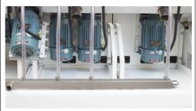
Optional grinding head drag plate lubrication function, to keep the grinding head smooth in the long period of use.
