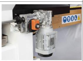
Automatically measure the glass thickness and adjust the position of the front pressing block to press the glass.
