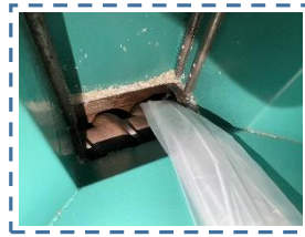
Screw feeds material into heating system
