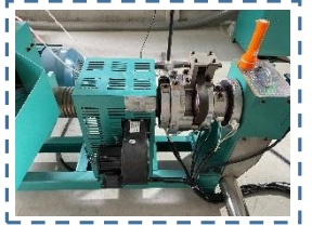
Heating to melt plastic
