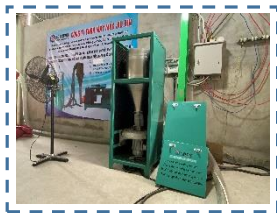
Cooling plastic granules with fan system
