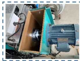
Direct hot cutting in the cutting chamber
