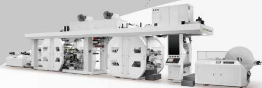
4+4 卫星式 • 双面阀口编织袋柔版印刷机 4+4 Colors CI Type Double Sides Valve Packetsflexographic Printing Machine
