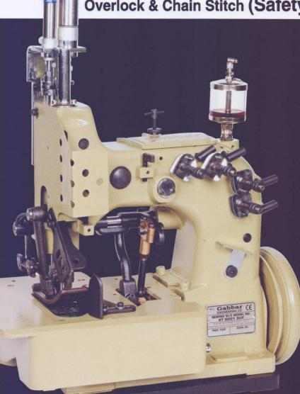
**Double Needle, Four Thread Combined Overedging and** Chain Stitch (Safety Stitch) **Sewing Machine with Lower Feed and Alternating** Upper Feed.
