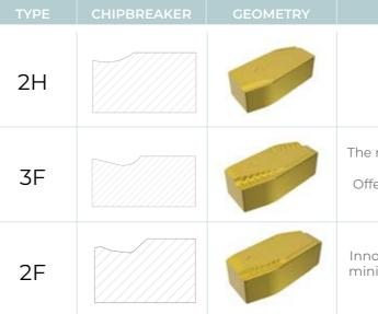
Another element not to be overlooked in choosing the chip-breaker is the average stock removal achieved. Chip-breakers are usually set to work halfway through the suggested removal range for the specific insert. If working continuously with removals at the limits of the characteristic range, an accurate choice has to be made, taking into account the chip section and the cutting force necessary to generate it.
