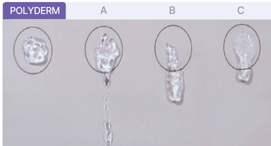
Photo of Viscosity test (after 4 mins, at 36.5°C) vertical Glass
