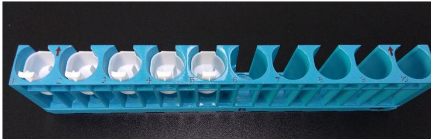
Fig. 4-39 Placement of QC Bottle Sleeves
