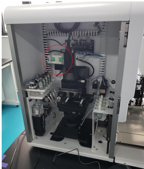
Fig. 5-7 Peristaltic pump position
