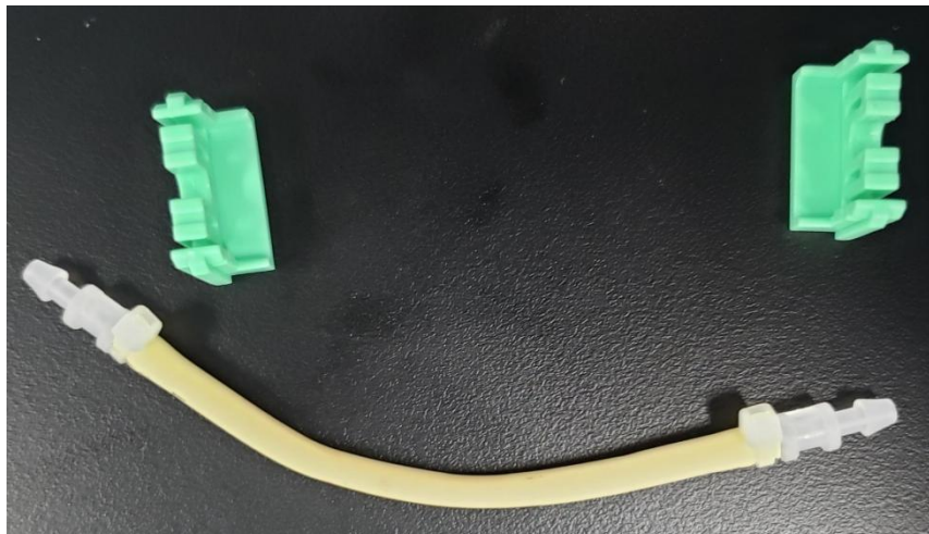
Fig. 5-13 Replace peristaltic pump tube
