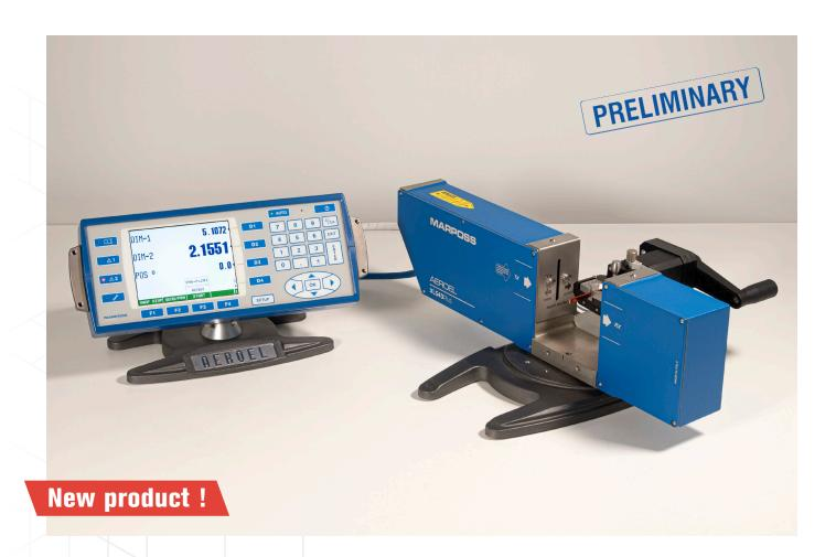
SUPER- WIRELAB.X40 is a high-performance tabletop laser micrometer to check off-line the rectangular wires.
