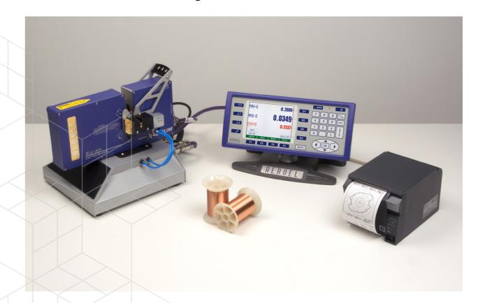
SUPER- WIRELAB.XY is a high performance tabletop laser micrometer designed to be used off-line to check diameter and ovalization of drawn or extruded products.
