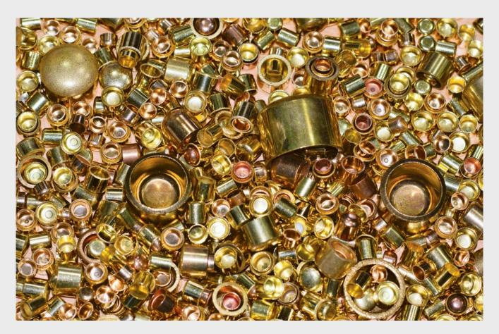
Various cartridge case cups and bullet jacket cups can be manufactured at desired standards at Altek Dokum facilities. Brass and tombac coils are brought ready for pressing after rolling, annealing and slitting processes.
