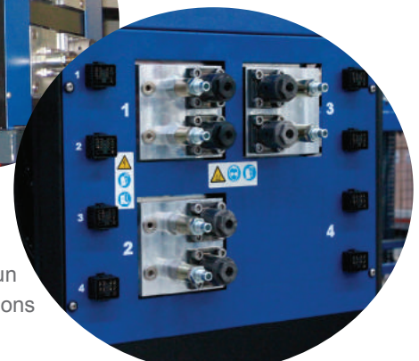
Easy access to pump manifolds
