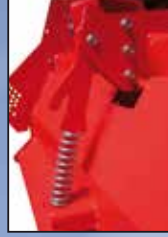
Yaylı arka kapak. With spring back cover.
