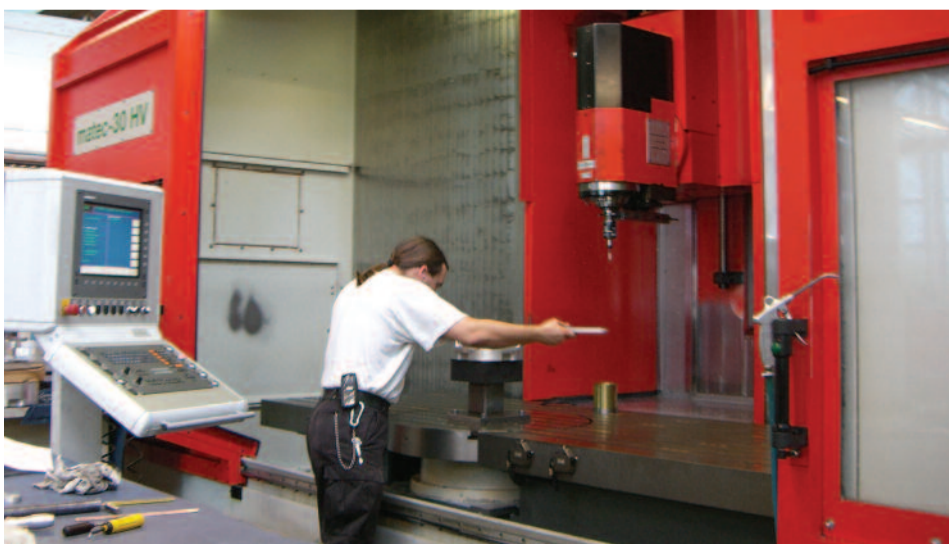
The 5-axis machining center matec-30 HV purchased in 2005 has proved its worth. The integrated off-center rotary table makes the machine ultra-flexible.
