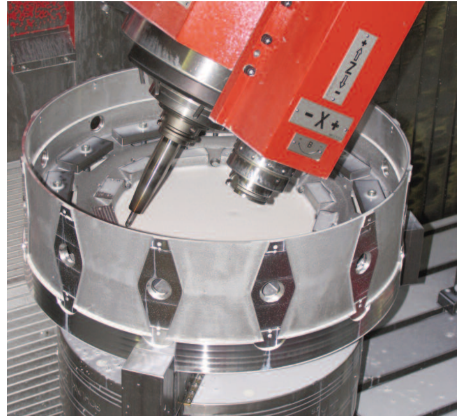
Above: Machining of a rotary table for automatic rotary indexing systems on the matec-30 FDZ. Material: cast aluminium. A special clamping system for extremely low locking pressure prevents the thin-walled parts from damage.
