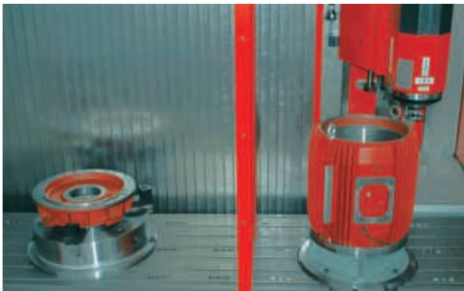
matec-30 HV 2 two separate working areas with rotary tables for pendulum machining
