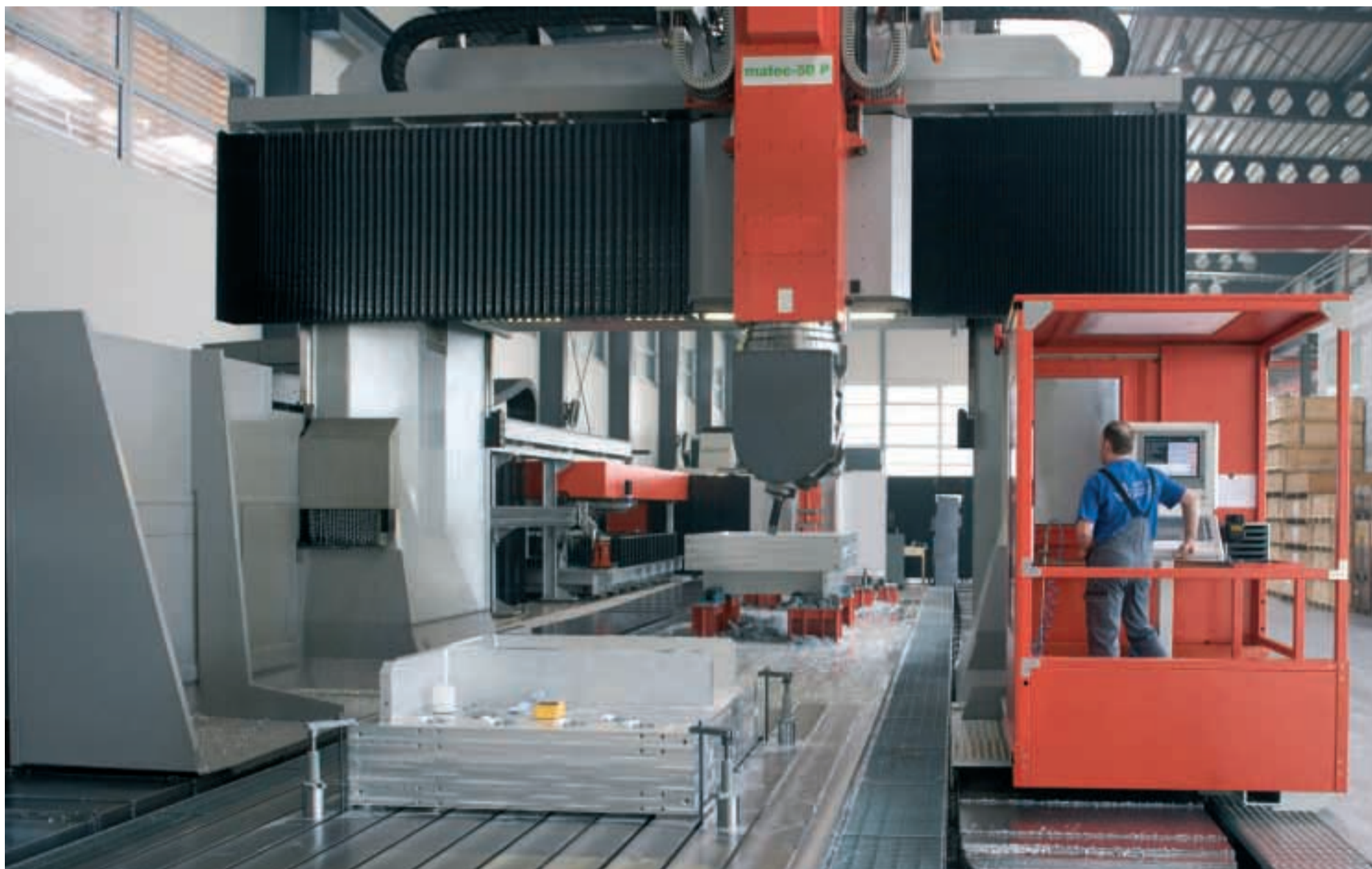
Customer-specific variant matec-50 P with 2-axis CNC motor spindle milling head and travelling operator platform X = 16 000 mm, Y = 5 000 mm, Z = 1 500 mm, W = 800 mm
