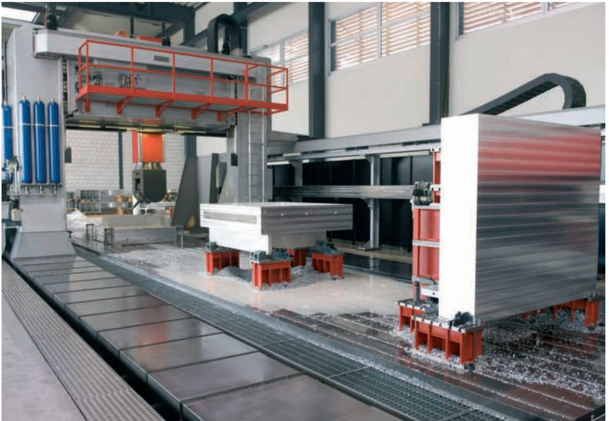
Customer-specific variant matec-50 P with 2-axis CNC motor spindle milling head and travelling operator platform X = 16 000 mm, Y = 5 000 mm, Z = 1 500 mm, W = 800 mm
