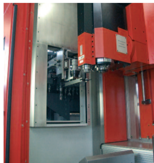
The tool magazine with 80 tools, fixed alongside the matec-30 FDZ, alternatively changes the tools into the motor spindle or the stationary spindle in front.
