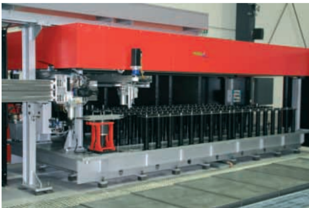
matec-50 P Tool magazine HSK 100 for 200 tools
