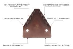
ALASKA SECTIONS ARE HEAT TREATED AND INDUCTION HARDENED / FULL HARDENED WITH HARDNESS OF 58-60 HRC
