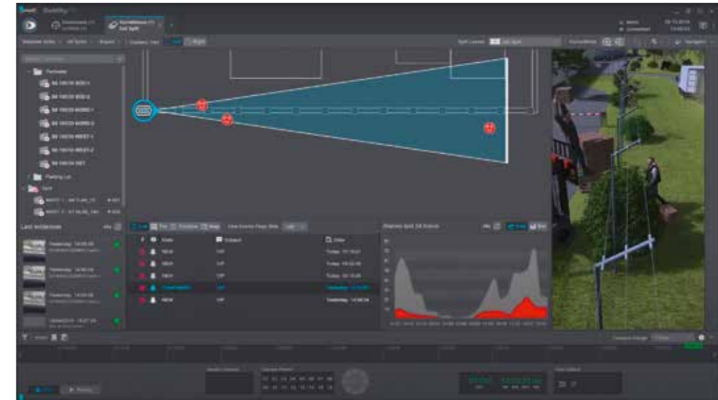
One of many examples of modern video analysis: AI-based object classification only forwards those alarms which really require human verification.
