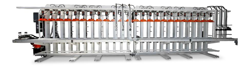
(Example of custom made, first generation MK1 Deck Art hydraulic press – max gluing width: 250 mm; max gluing length: 7680mm)
