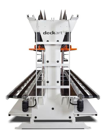
It is a well-known fact that the cold wood lamination process is the best possible way of ensuring the quality and durable bonding of wood using adhesives. With Deck Art cold hydraulic presses, you will achieve the finest quality of lamination of the flooring hardwood wear layer to the flooring core, and ensure a perfectly stable base for further processing with no effort.
