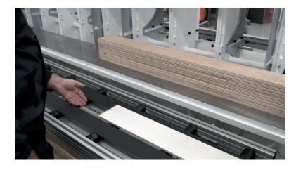
**Specially designed, adjustable back supports** will keep the material centered for even pressure distribution, this gives you maximum flexibility when gluing different widths of flooring on a single press.
