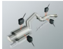
Vibration test of high-temperature-muffler
