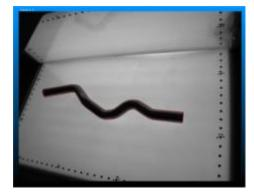
The cameras are triggered synchronously. Nevertheless, operator should avoid any motion blur effects due to moved or post-oscillating tubes. The pictures are transferred to the computer's RAM for further processing in
