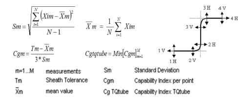
**TubeInspect P16.2, P16.2 HRC:** Verification of the specified measuring accuracy is considered fulfilled when the Cgk value  $\ge$  1.33 for the sheath tolerance characteristic at a tolerance of T = 0.85 mm has been obtained with the TubeInspect Master Tube.
