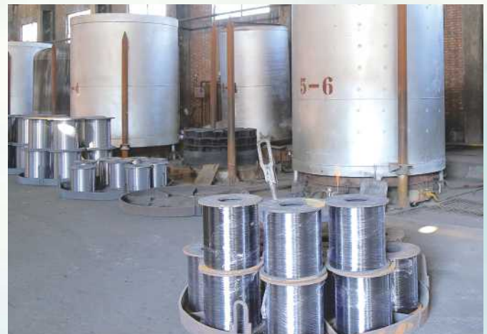
Annealed with shielding gas (Oxygen Free Annealed)
