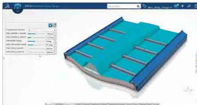
Figure 1: Floor panel design
