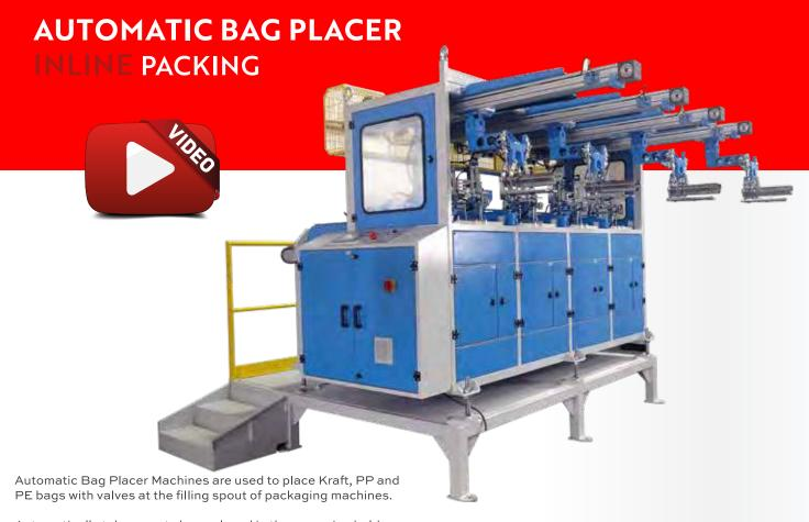
Automatically takes empty bags placed in the magazine holder as bundles, opens the valve mouth, and installs it on the spout of the filling machine.
