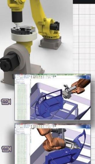
Collision control; Control of additional axes of the robotic cell. The Robot control program is generated taking into account the currently selected robot type. SprutCAM outputs the technological commands inherent to the selected robot type within the created control program.
