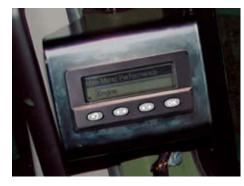
**Monitoring Systems.** The D7R-II dozer maximizes on-board diagnostics capability using electronic control modules (ECMs) to monitor engine and machine (transmission, hydraulic and brake) systems. Cat Electronic Technician (ET) software accesses
