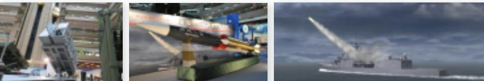
The Hsiung /Feng III (HF III) is one of the world's most compact supersonic anti-ship missiles featuring advanced design of integrated rocket ramjet (IRR) capable of long range flight with small size and lightweight. With a precise flight control system, the HF III can fly at sea-skimming altitude and, the warhead having remarkably armor-piercing capability, it generates tremendous destructive power when hitting the target. The HF III is currently in service with the ROC Navy.
