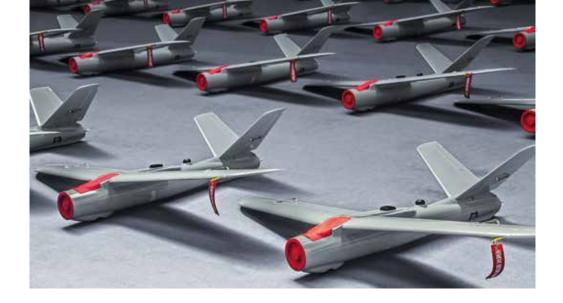
The complete WARMATE set is composed of three air vehicles (AVs), 3 warheads, a lightweight ground control station (GCS) and a ground data transceiver, which allows for the user to control the AV, and receive real time video. The system can be packed into two ruggedized backpacks and carried by two users.
