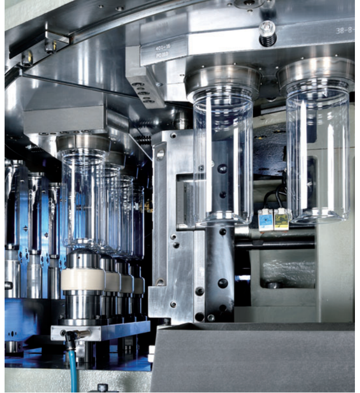
Easy access to blow station enables additional functionality and fast mold change
