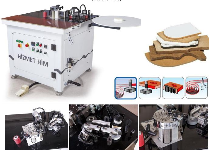
**Description:** Curved edge banding machine tool is used in the furniture sector for serial and uniform coating with skirting tape (PVC edge, etc.) straight, convex and concave edges of the wooden profiles used for the production of furniture.
