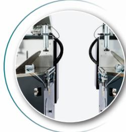
Compound cuts (pivoting and tilting) on both heads (45° x 45°)
