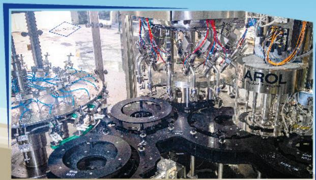
Suitable for hygienic conditions The machine environment and the upper ceiling are completely closed, and HEPA filtered fans create positive pressure to prevent dust or bacteria from entering the machine.
